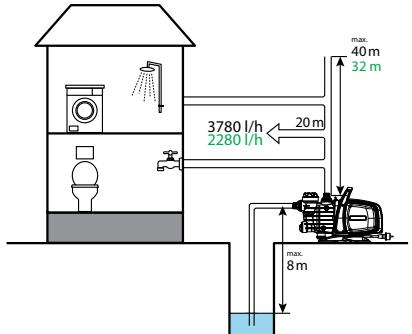
**GB** Electronic self-priming gardening pump with automatic ON/OFF and dry run protection. Also suitable for the pressurisation of water in domestic applications. Compact, light, robust and easy to use. Equipped with orientable suction connection plus integrated non-return valve and pre-filter for extended pump life. Facility to empty residual water to protect it from frost and accumulation of lime scale also included.
